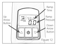
return to standby mode without saving the new setting, press and release the *Start/Stop Button* momentarily instead of holding it down.
