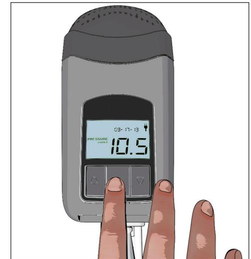
**NOTE for Z1:** The *Auto Stop Feature* will stop the therapy if a large air leak is detected between the Z1 outlet and the mask. This may also happen at times when the mask is not being worn properly. This common condition should be resolved once all connections are secure, the mask is properly worn, and the *Start/Stop Button* has been pushed.
